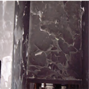
Delaminated paint that has burned in a fire. Courtesy of Exova Warringtonfire.
